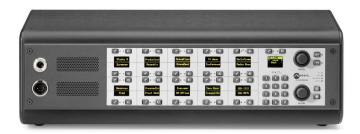
The IC.20D is the desktop version of the IC.20 rack-mount station we showed you earlier. The 20 station preset locations are equipped with high-resolution OLED displays; the OLED callback window and dialing pad let operators call any station not programmed to a preset location. Naturally there's a built-in speaker, front-panel 4-pin locking headset jack, front-panel mic input, an Ethernet port for fast hookup, and internal auto-sensing power supply.
